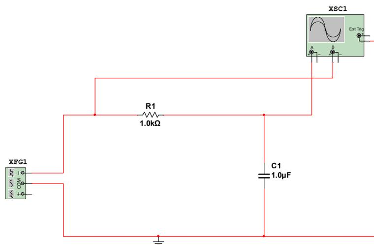
Fig. 2 A Low Pass Filter using MultiSim
