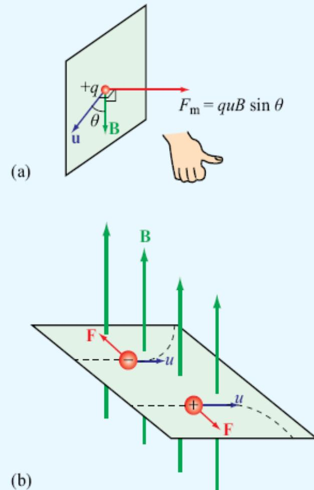
**Figure 5-1** The direction of the magnetic force exerted on a charged particle moving in a magnetic field is (a) perpendicular to both  $\mathbf{B}$  and  $\mathbf{u}$  and (b) depends on the charge polarity (positive or negative).
