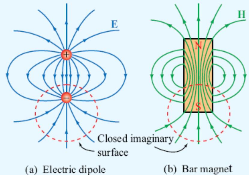
**Figure 5-15** Whereas (a) the net electric flux through a closed surface surrounding a charge is not zero, (b) the net magnetic flux through a closed surface surrounding one of the poles of a magnet is zero.
