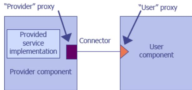
Figure 3. Provider and user proxies. The user component only needs to know the service interface and gets the proxy code that runs the provided service.
