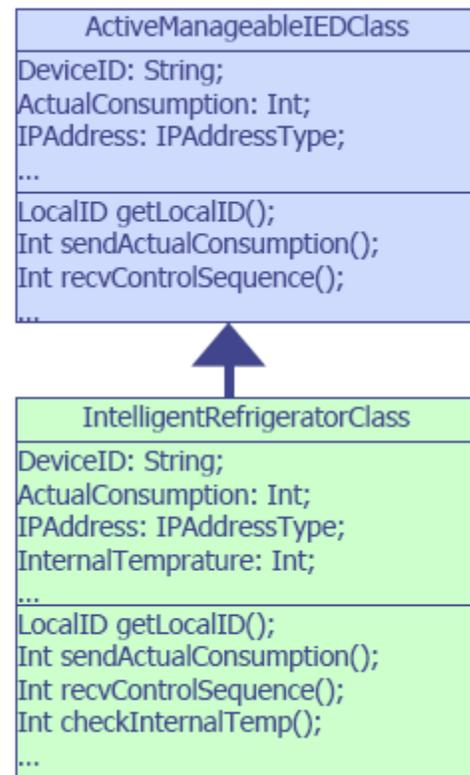
Figure 5. UML class diagram: Deriving the intelligent refrigerator class from the active manageable device class.
