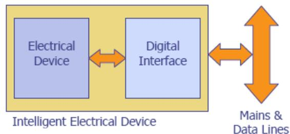
Figure 1. An intelligent electrical device is connected through an interface that embeds control and communication logic.
