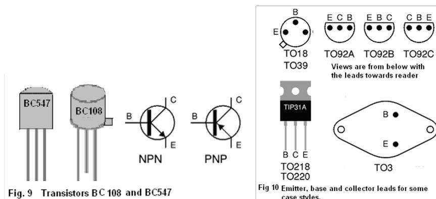
Their most important specifications includes  $I_C$  (collector current),  $V_{CE}$  (collector to emitter voltage) ,  $h_{fe}$  (h parameters) and power rating.
