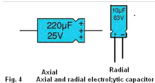
attached to each end (220  $\mu\text{F}$ ) and (ii) Radial, where both leads are at the same end (10  $\mu\text{F}$ ).
