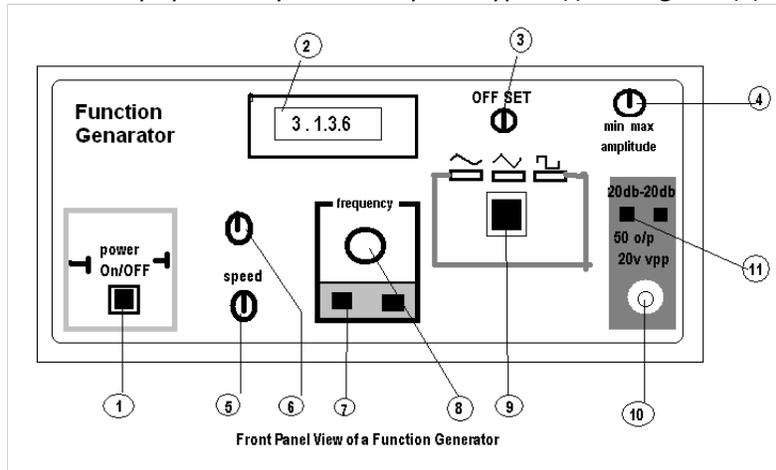
Some of the front panel controls of a typical function generator are:
