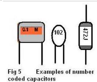
Any letters just indicate tolerance and voltage rating. For example, 102 means  $10 \times 10^2 \text{ pF} = 1 \text{ nF}$  and 472J means  $4700 \text{ pF} = 4.7 \text{ nF}$  (J means 5% tolerance).
