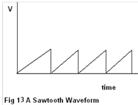
This is a voltage that changes continuously and linearly with time. When it reaches a predefined value the ramp is reset. When a trigger event is recognized the reset is released, allowing the ramp to increase again. The time base voltage usually drives the horizontal amplifier. Its effect is to sweep the electron beam at a constant speed from left to right across the screen, then quickly return the beam to the left in time to begin next sweep.
