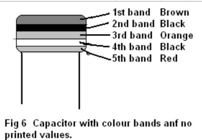
For example: Brown, Black, Orange means  $10,000 \text{ pF} = 10 \text{ nF} = 0.01 \mu\text{F}$ .
