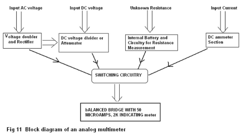
Fig 11 Block diagram of an analog multimeter
