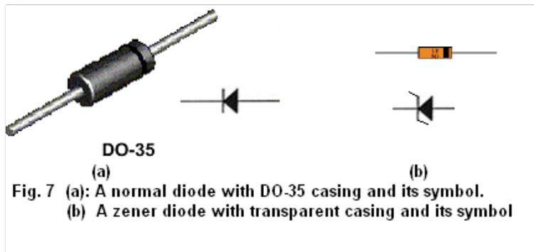
Other diodes may be made by a p type or n type semiconductor and a metal. If the junction is made between a metal and a semiconductor then it is called a Schottky Diode, whose application is in rectifying and non-rectifying contacts. If the PN junction is made between very heavily doped materials then it forms a Zener Diode. These are used for voltage regulation in power supplies and have breakdown voltages which are very low. The normal diode has a breakdown voltage of greater than 100V.
