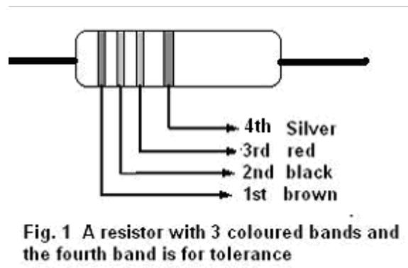
The first two bands near an end indicate first 2 digits, digit corresponds to 3<sup>rd</sup> band is the power of 10 to be multiplied and 4<sup>th</sup> band indicates tolerance as mentioned in the table. Refer to figure 1, where brown = 1, black = 0, red = 2 and silver = 10% tolerance. Hence, its value is  $10 \times 10^2 \Omega = 1 \text{ k}\Omega$ .
